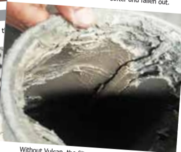
Without Vulcan, the filter was quickly stuck by scale deposits, and it had to be changed every 48 hours.
