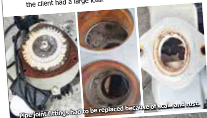
Pipe joint fittings had to be replaced because of scale and rust.
